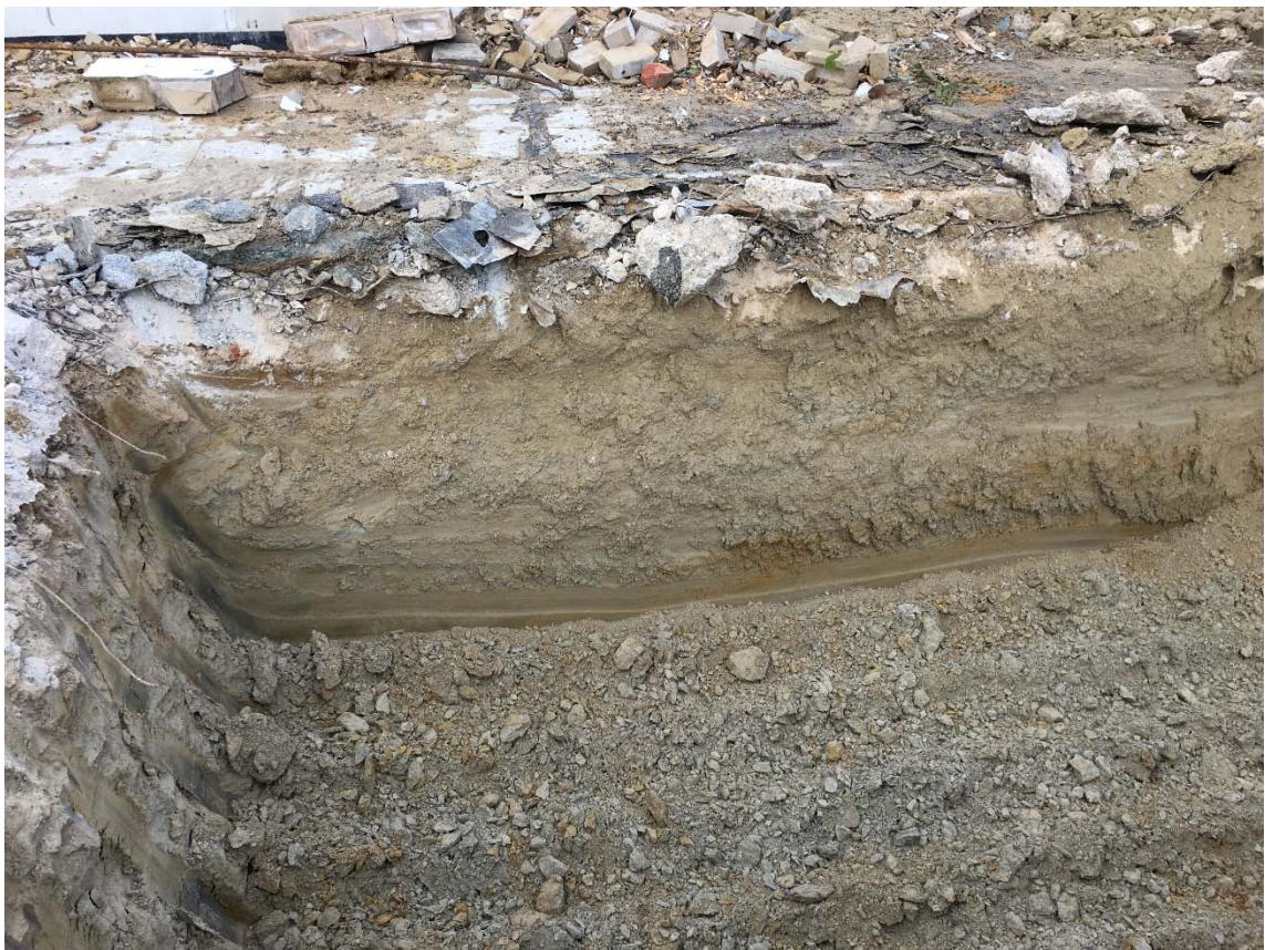
Figure 4: Trial Pit TP2 photograph, Goldsel Road, Swanley, Kent. Trench depth here is 0.8m.
