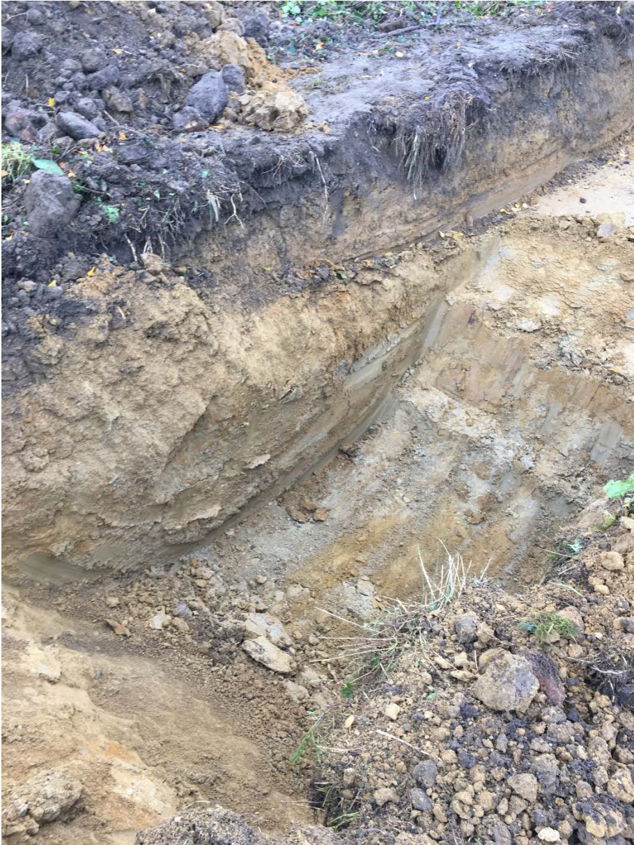
Figure 10: Trial Pit 9 photograph, Goldsel Road, Swanley, Kent. Trench depth here is 1.8m.
